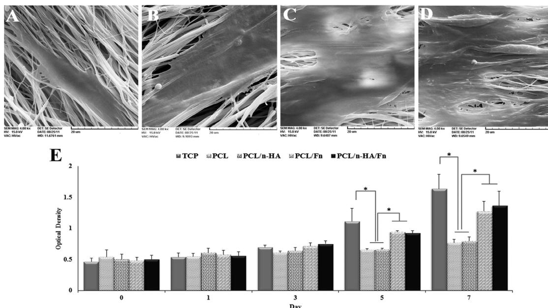
**Figure 3.** Investigation of MSC adhesion and proliferation by SEM on (A) PCL, (B) PCL/nHA, (C) PCL/Fn and (D) PCL/nHA/Fn scaffolds or by MTT assay on (E) scaffolds and TCPS during a 7-day culture period. Scale bars with their magnifications are given in the figures. Asterisk shows significant difference with  $p < 0.05$ .
