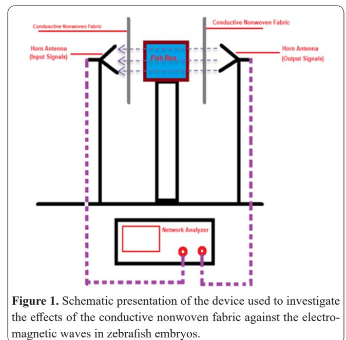
**Figure 1.** Schematic presentation of the device used to investigate the effects of the conductive nonwoven fabric against the electromagnetic waves in zebrafish embryos.
