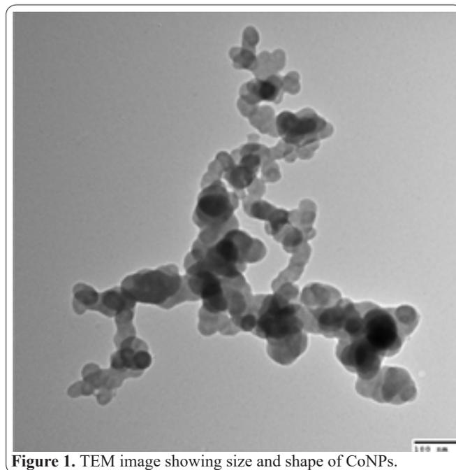
**Figure 1.** TEM image showing size and shape of CoNPs.
