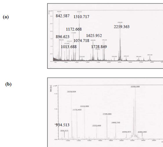
**Figure 6.** Peptide Mass Finger Print of ricin. In-gel tryptic digest of (A) native and (B) denatured ricin in the reflectron mode using CHCA as matrix.
