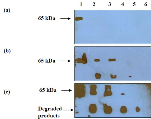
**Figure 4.** Western blots of native and denatured ricin X-ray film exposed for (A) 10 min; (B) 90 min; (C) 180 min. Lanes: 1) Native ricin; 2) 3.75 min denatured ricin; 3) 7.5 min denatured ricin ; 4) 15 min denatured ricin; 5) 30 min denatured ricin; 6) 60 min denatured ricin.
