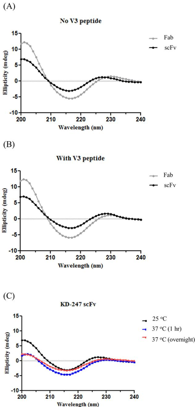
**Figure 5.** Far-UV circular dichroism (CD) spectra to evaluate secondary structures. The refolded KD-247 scFv (black) was compared to KD-247 F<sub>ab</sub> (grey) in the absence of V3 peptide (A) and in the presence of V3 peptide (B). (C) CD of the refolded scFv at 25 °C (black), after 1 hour incubation at 37 °C (blue) and after overnight incubation at 37 °C (red).
