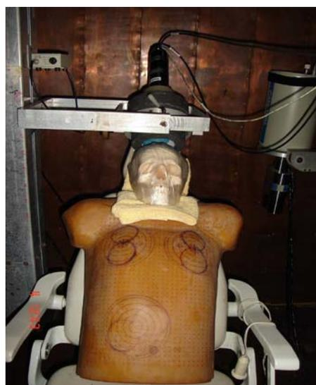
**Figure 2.** Brain phantom inserted in the resin skull positioned for the measurements
