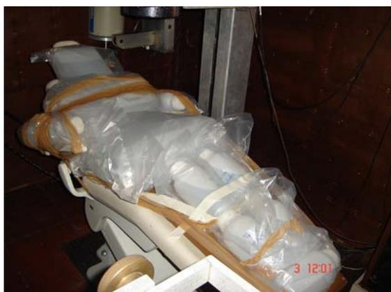
**Figure 1.** Whole body phantom positioned for the calibration in the IRD whole body counter
